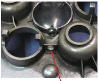
You will need to drill access holes for the screwdriver to set the sheet metal screws in the acorn.
